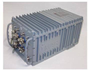
interfaces like Ethernet, RS422, MIL-STD-1553B and CAN, internal data storage and position accuracy on sub-decimeter level.
